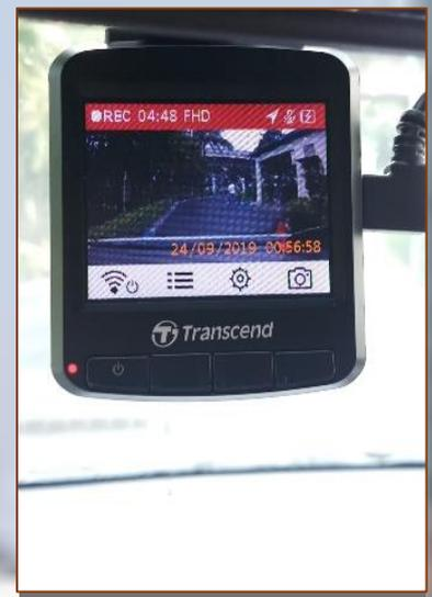
*A vehicle-mounted dashboard camera, recording the road conditions*
