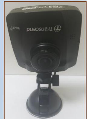
*A typical dash board camera, with a vacuum cup below to easily mount on a vehicle*
